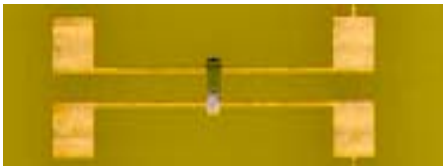
Figure 6: Component shifted 180µm in Y-direction
