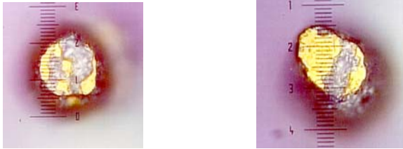
Figure 16: Insufficient ICA underneath the Au-stud bump
