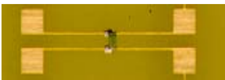
Figure 5: Component shifted 200µm in X-direction
